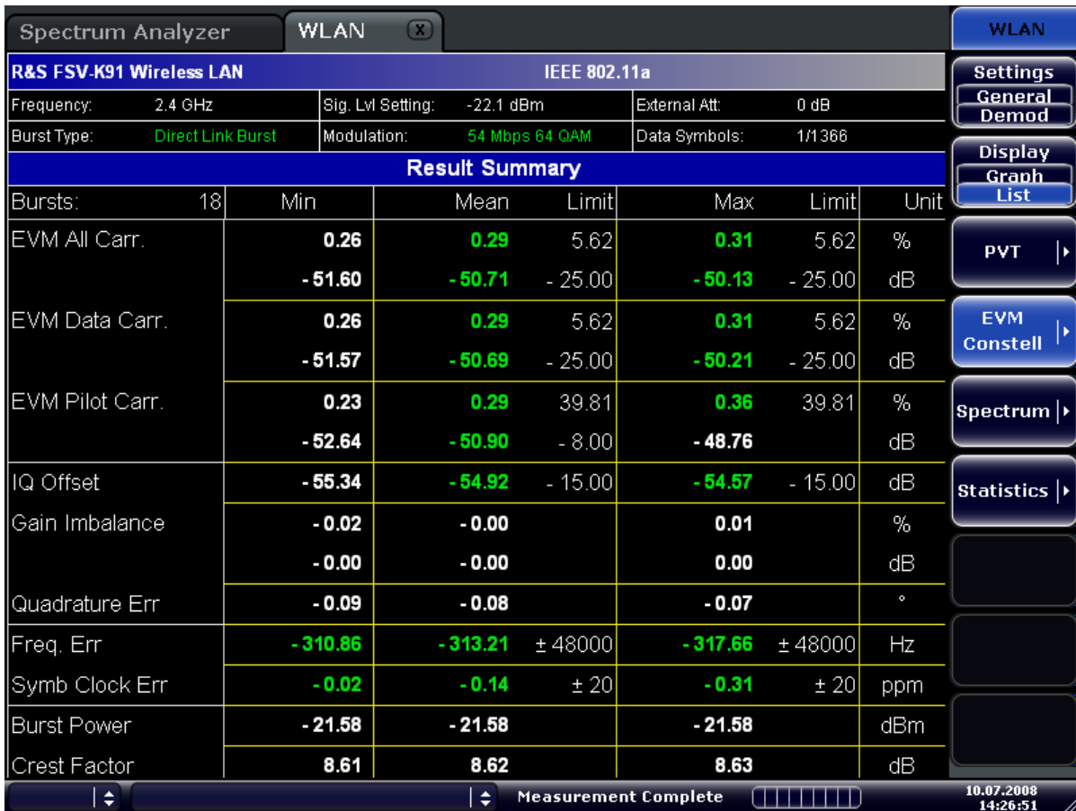
Fig. 4-5: Result summary list for measurements on OFDM signals
