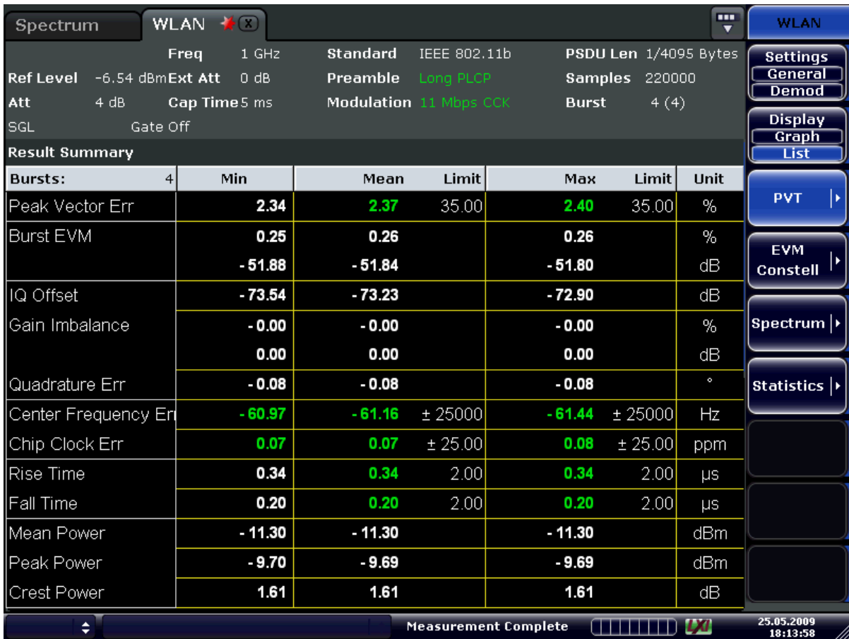
Fig. 4-6: Result summary list for measurements on DSSS/CCK/PBCC signals
